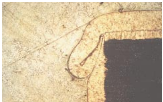
G-42 Plating fold, inclusion, and nodule
