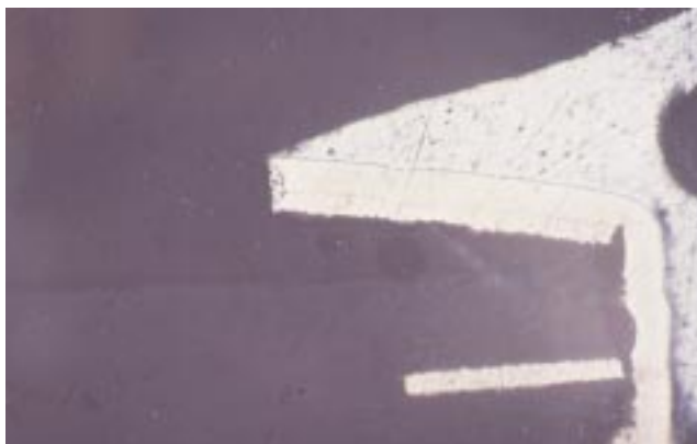
G-9 Lifted land Innerlayer separation Poor plating adhesion to hole wall Separation along vertical edge of external land
