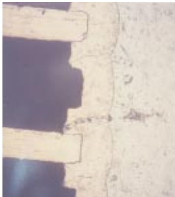
G-32 Flex barrel crack
