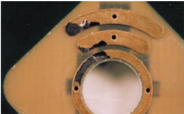
D-8 Gold plating adhesion failure
