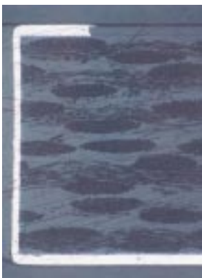
P-9 Typical flush microsection
