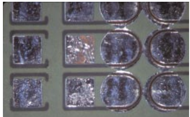
E-12 Solder dewetting and nonwetting surface lands
