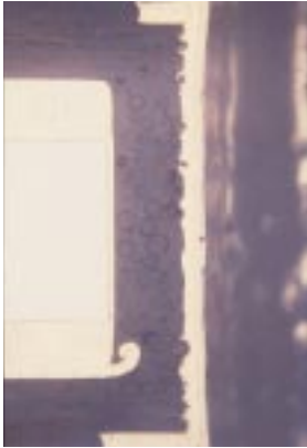
P-7 Burr on metal core
