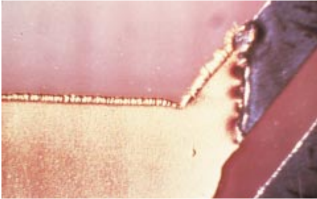
D-7 Gold contacts Plating anomalies
