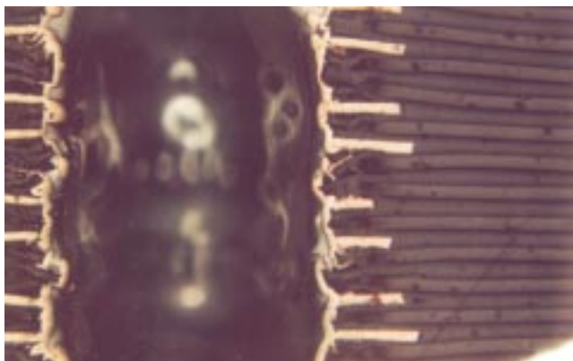
G-33 Flex plating voids
