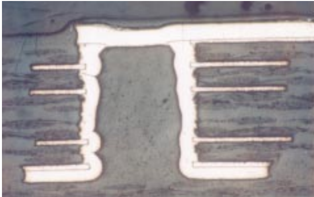
F-7 Surface misregistration in blind via
