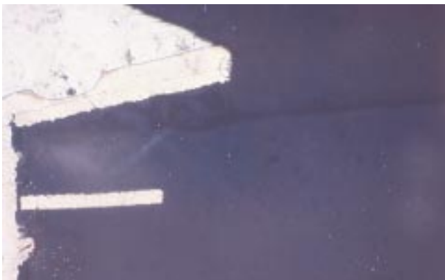
C-21 Severe lifted land, corner crack, innerlayer separation
