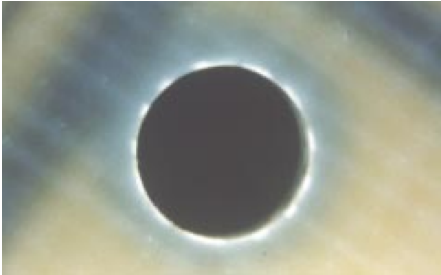
B-1 Unsupported hole Haloing
