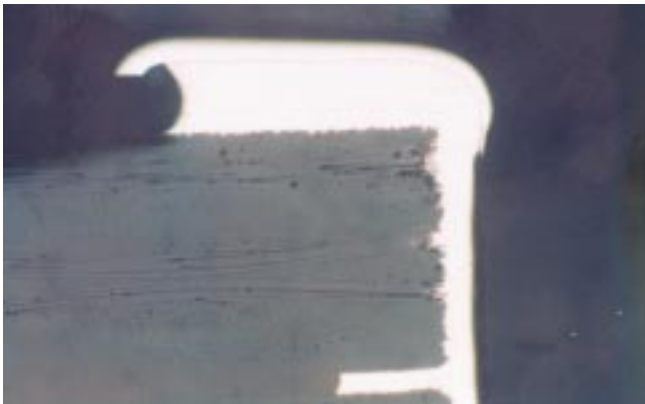
C-8 Conductor overhang
