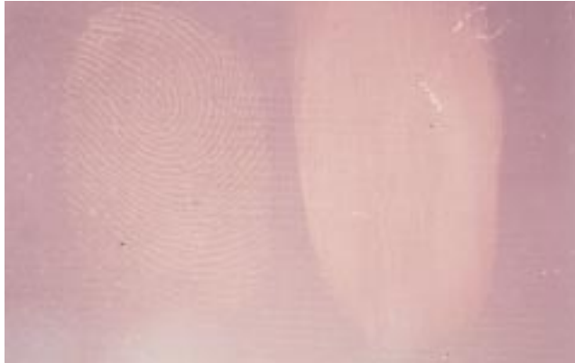
A-1 Fingerprint on copper foil (left side) Smudge (right side)
