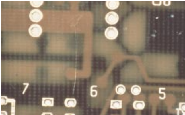
M-2 Wrong layup, multilayer board
