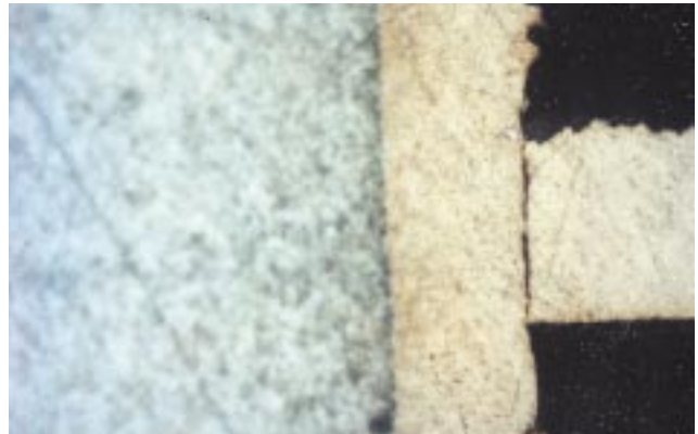
G-5 Innerlayer separation
