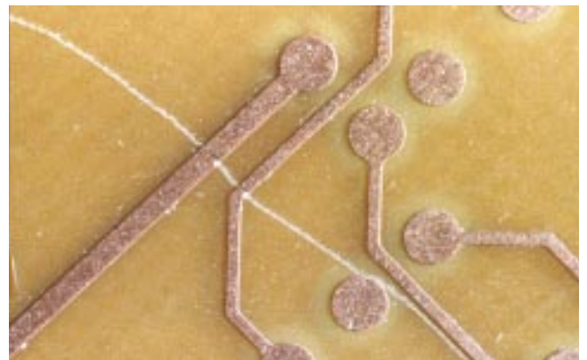
C-17 Scratched innerlayer conductors and substrate
