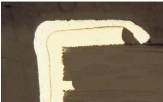
C-9 Conductor undercutting collapse
