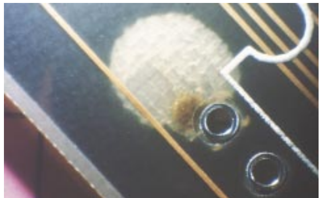
B-24 Blistering adjacent to land Delamination
