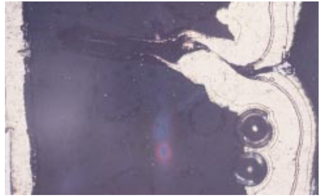
P-5 Void in backfill dielectric material of metal core board Plating crack
