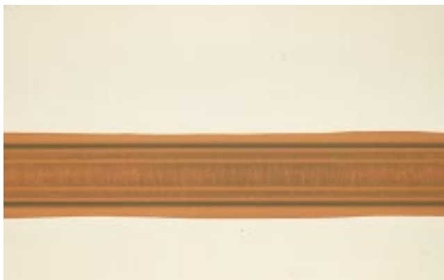
N-3 Poor trimming
