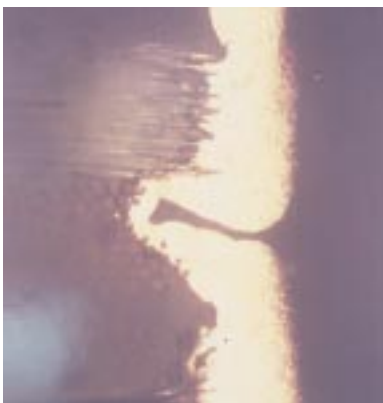
G-15 Thin area in copper plating
