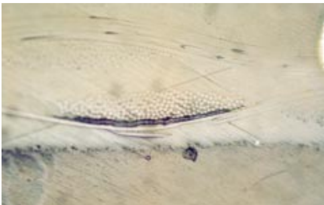
B-14 Measle (Cross-section)
