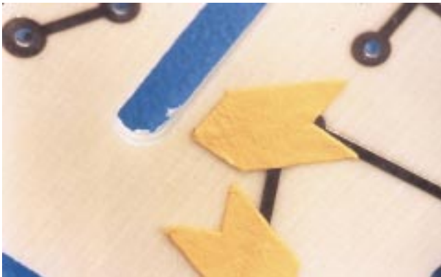
H-2 Slot (protruding fibers)
