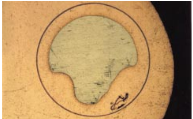
G-47 Horizontal microsection Plating anomaly
