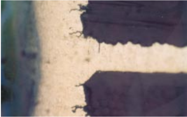
G-1 Internal foil crack Plating cracks (barrel)
