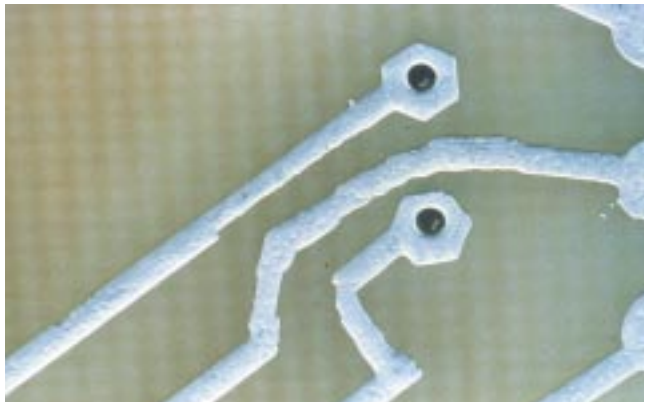
C-2 Conductor width reduction Rough edge definition
