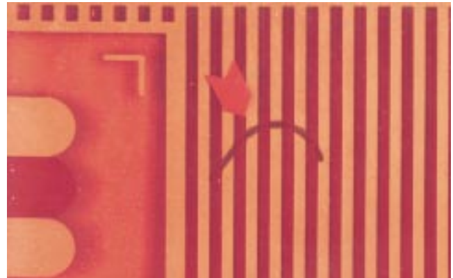
N-11 Foreign material in covercoat
